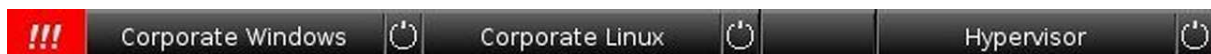
Fig. 3: OpenTC taskbar (cropped) with a red button indicating that the TCB is not in a known state and that unsealing the image has not been possible.
